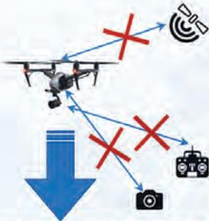
Isolates the UAV forcing it to perform an emergency landing on the position where it loses the connection.
