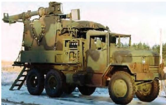
Figura 2 – Sistema RADAR AN/MPQ 49B FAAR.
